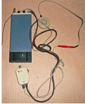
Basic remote control unit. This variation had neither a built-in loudspeaker nor a vibrator unit.
