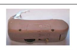
An inconspicuous wireless (induction loop principle) 'behind-the ear' hearing aid type earphone was developed in the GDR for the PR-35 and the PR-36. It was probably imported and used in Czechoslovakia.
